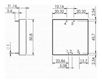
An additional frame with a height of 1 mm can be attached to seal the housing with the potting.
